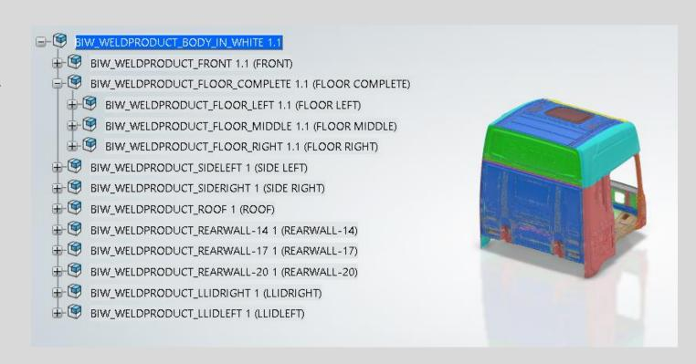
In picture Doors missing and Rear Wall have ben divided in 3 separate components to manage the different lengths
